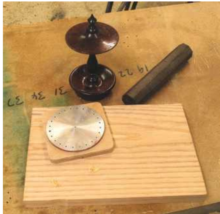
▲ Pic.2 A finished earring tidy and the wood needed, two pieces of 80 x 80mm ash planed 15mm thick, a piece of contrasting timber like this ebony 125mm long by 20mm square
